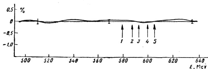
Dependence of the quantity  $[\sigma(E) - \bar{\sigma}(E)]/\bar{\sigma}(E)$  on the proton energy  $E$ . The thresholds of the reactions  $pp \rightarrow pp\pi^0\pi^0(1)$ ,  $pp \rightarrow d\pi^0\pi^+(2)$ ,  $pp \rightarrow pn\pi^0\pi^+(3)$ ,  $pp \rightarrow pp\pi^+\pi^-(4)$ , and  $pp \rightarrow nn\pi^+\pi^+(5)$  are indicated by arrows.
