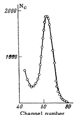
FIG. 2. Portion of the spectrum of  $\gamma$  rays around 1.64 Mev with total absorption peak, taken for  $E_p = 2.72$  Mev.
