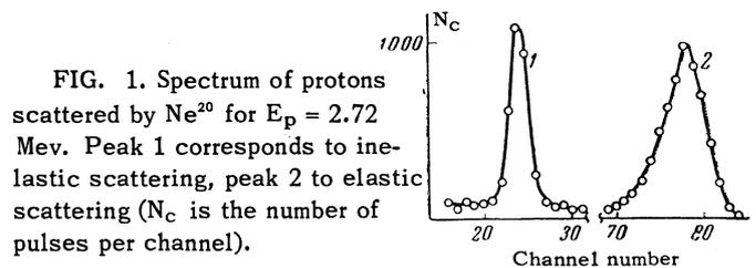
FIG. 1. Spectrum of protons scattered by  $\text{Ne}^{20}$  for  $E_p = 2.72$  Mev. Peak 1 corresponds to inelastic scattering, peak 2 to elastic scattering ( $N_c$  is the number of pulses per channel).
