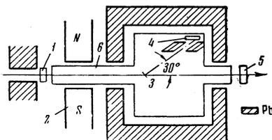
FIG. 2. Experimental setup. 1, 5 - ionization chambers, 2 - magnet, 3 - target, 4 - nuclear emulsion, 6 - vacuum chamber.
