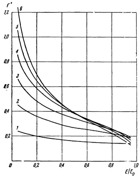
FIG. 4. The  $\Gamma'$  curves correspond to the following values of  $t$ : 1-0.2, 2-0.4, 3-0.6, 4-0.8, 5-1.0, 6-1.2.
