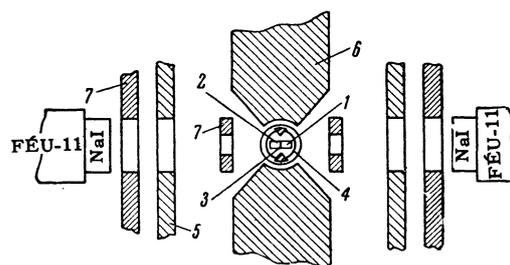
Schematic of the experimental apparatus: 1 – sample of enriched Zn, 2 – sample of normal Zn, 3 – face of enriched sample, irradiated at cyclotron, 4 – shield at 80°K, with Armco iron pole pieces, 5 – magnetic shield (iron), 6 – pole of electromagnet, 7 – lead collimators. Samples 1 and 2 were soldered to the bottom of a container of liquid helium. The photomultipliers were surrounded by a permalloy screen 5 mm thick.
