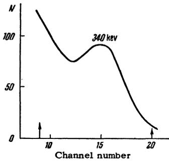
FIG. 1. Spectrum of scattered  $\gamma$  rays from  $\text{Nd}^{147}$  (the arrows show the window of the discriminator).
