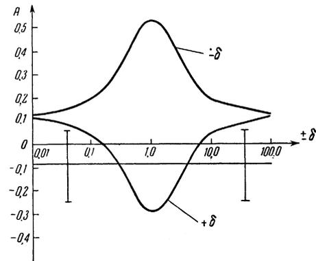
FIG. 3. The asymmetry coefficient  $A$  in  $\beta\gamma$  correlation with circularly-polarized  $\gamma$  rays as a function of  $\delta$ , the amplitude ratio  $E2/M1$ .
