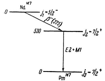
FIG. 2. Decay scheme for the transition  $\text{Nd}^{147} \rightarrow \text{Pm}^{147}$ .
