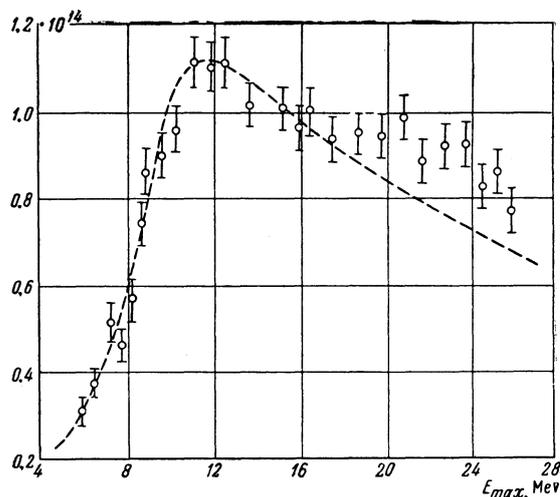
FIG. 1. Yield of the reaction Rh<sup>103</sup>( $\gamma, \gamma'$ )Rh<sup>103m</sup> at various maximum x-ray energies  $E_{\max}$ . Ordinates – saturated activity per second per mole per ampere of ionization current of the absolute chamber. The dashed curve is the yield curve calculated under the assumption that the reaction cross section is zero at energies above 12.5 Mev.
