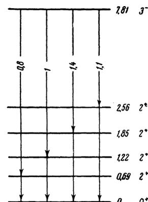
FIG. 2. Proposed scheme of levels and two-cascade  $\gamma$  transitions of  $\text{Nd}^{144}$ . The numbers on the arrows indicate the relative intensities (the energies of the corresponding levels are in Mev).
