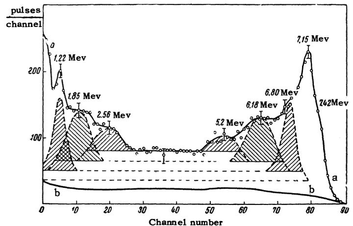
FIG. 1. a — Coincidence spectrum of captured  $\gamma$  radiation of  $\text{Nd}^{144}$ , occurring when the capture is in the energy range 1–8 Mev (rms errors); b — spectrum of random coincidences under the same conditions.
