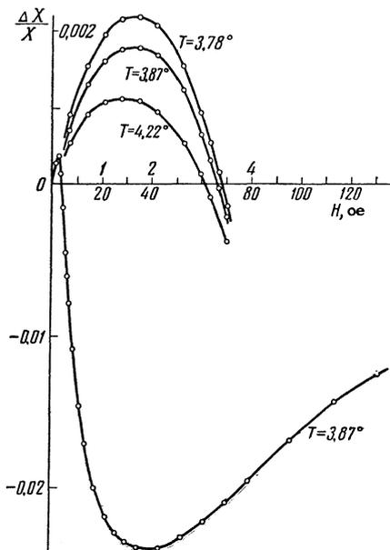
netic field which was parallel to the axis of the coil and the specimen. Along the ordinate axis is plotted the relative change of the reactive component of the impedance relative to the total magnitude, the latter being determined from the change in the oscillator frequency when the sample has passed into the superconducting state. In the top portion of the diagram are plotted the first parts of the curves at various temperatures on a larger scale.
