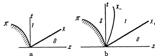
FIG. 1. Waves produced in the motion of the piston: a - in ordinary hydrodynamics, b - in magnetohydrodynamics. 1 - line of motion of piston; X - characteristic in ordinary hydrodynamics,  $dx/dt = v_x + c$ ;  $X_+$  - 'fast' characteristic in magnetohydrodynamics,  $dx/dt = v_x + U_+$ ;  $X_-$  - 'slow' characteristic in magnetohydrodynamics,  $dx/dt = v_x + U_-$ ; 0 - standstill region; 1 - simple wave; 2 - non-simple wave.
