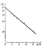
As can be seen from the diagram a decrease in the intensity of the satellites occurs as a result of plastic deformation. It must be emphasized that the width of the "total" line remains, within experimental error, the same as for undeformed samples.
