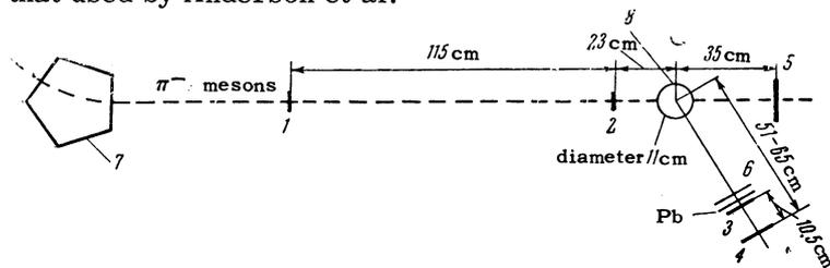
FIG. 1. Geometry of the charge-exchange scattering experiment: 1, 2 – scintillation counters 6 x 6 cm; 3, 4, 5 – scintillation counters 12.6 x 11.5 cm; 6 – scintillation counter 16 x 17 cm; 7 – deflecting magnet; 8 – liquid hydrogen.
