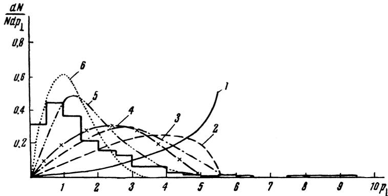
FIG. 5. Transverse-momentum distributions obtained under the assumption that the mesons are monoenergetic ( $p_0 = 5.7$ ). Curves 1 to 6 correspond to  $n = 0, 1, 2, 3, 10,$  and  $16$ .
