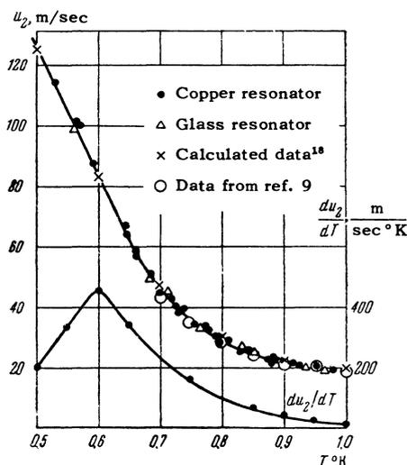
FIG. 3. Dependence of second sound velocity upon temperature.
