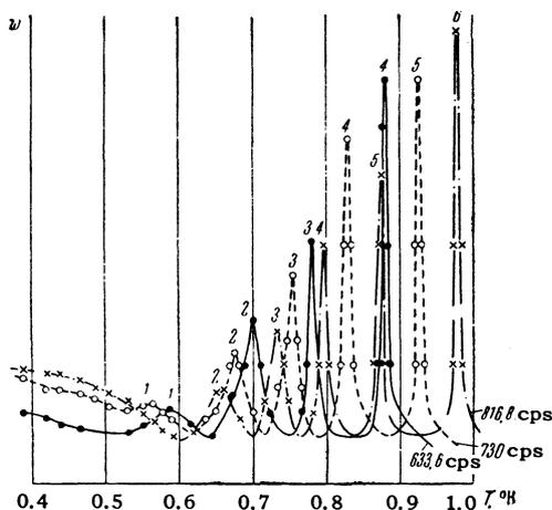
FIG. 2. Dependence of amplitude of second sound oscillations in resonator upon temperature. Number of resonances indicated by numbers on curves. Frequency and current supplied to heater held constant.
