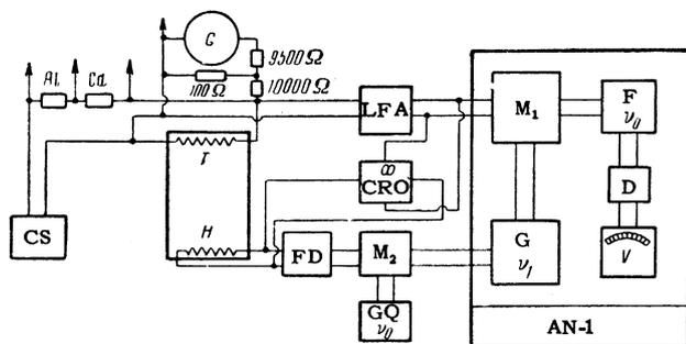
FIG. 1. Diagram of apparatus for observation of second sound (for symbols, cf. text).
