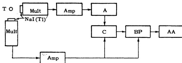
FIG. 1. Block diagram of the luminescence coincidence spectrometer: M – target, Amp – amplifier, A – amplitude analyzer, C – coincidence circuit, BP – bandpass filter, AA – 20-channel amplitude analyzer.
