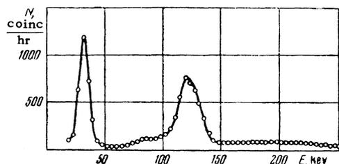
FIG. 3. Spectrum of coincidence pulses with 63-keV  $\gamma$  line.
