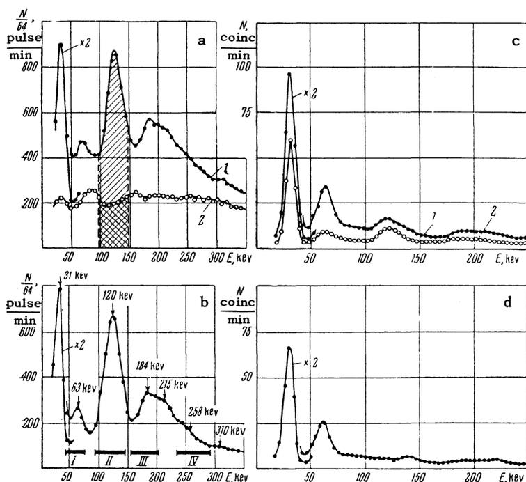
similar to the spectrum of the pulses in the channels. Each measurement of the spectrum of the total number of coincidences was accompanied by measurement of the spectrum of the random coincidences. The desired spectrum of true coincidences was obtained by finding the difference of these two successively measured spectra. In what follows only the spectra of the pure coincidences will be discussed.
