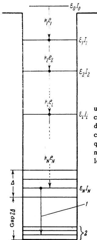
FIG. 1. The cascade scheme used in the estimation of the circular polarization and angular distribution of quanta from (ny) capture. 1 is the characteristic quantum in the  $\gamma$  spectrum of the n-capture; 2 represents the collective excitation of the nucleus.
