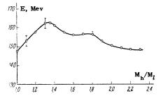
FIG. 4. Dependence of the most probable total kinetic energy of Th<sup>232</sup> fission fragments on the fragment mass ratio (the statistical errors are indicated).
