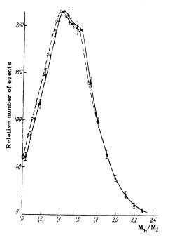
FIG. 2. Fission probability as a function of the mass ratio of the fragments: O - uncorrected data,  $\bullet -$  corrected for dropping of neutrons.
