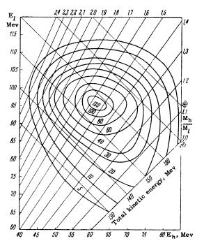
FIG. 1. Contour map of Th<sup>232</sup> fission by 14.9-Mev neutrons. The subscripts h and l refer to heavy and light fragments respectively.
