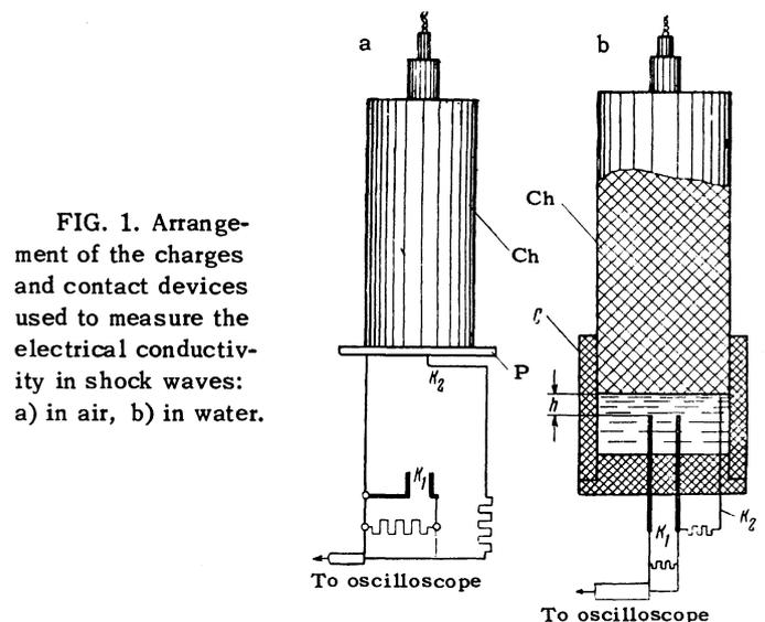
FIG. 1. Arrangement of the charges and contact devices used to measure the electrical conductivity in shock waves: a) in air, b) in water.
