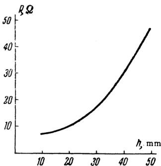
FIG. 3. The resistance  $R$  in a shock front in water as a function of the distance  $h$ .
