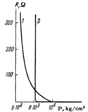
FIG. 4. The resistance  $R$  in a shock front as a function of pressure: curve 1 is for paraffin and curve 2 for Plexiglas.
