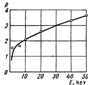
FIG. 4. Ratio of maximum density of deposit  $P_c$  in the central patch (corresponding to the [100] direction) to the maximum density of the positive  $P_s$  in the side patches (corresponding to the [110] directions) as a function of the energy of bombarding ions,  $E$ .
