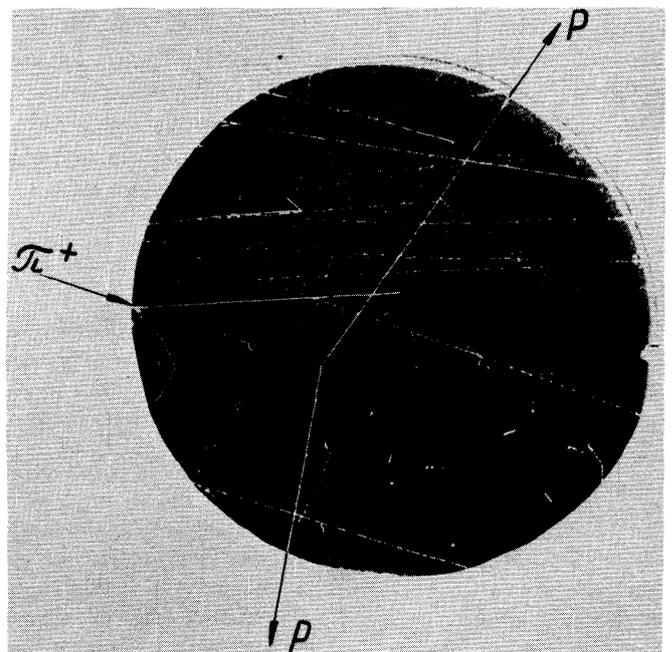
FIG. 1. Two-pronged star resulting from the absorption of a  $\pi^+$  meson by a carbon nucleus.
