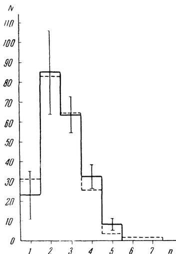
FIG. 3. Distribution of stars by number of prongs.  $N$ —number of stars,  $n$ —number of prongs in the stars. The solid line is the results of the present work, the dotted line is the data obtained in reference 11 for 115 stars produced in the absorption of 250-270 Mev energy  $\pi^+$  mesons by carbon nuclei.
