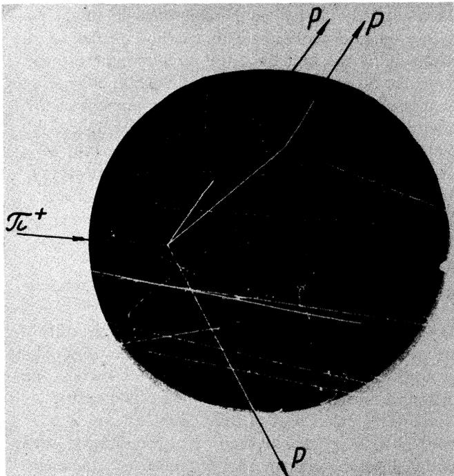
FIG. 2. Three-pronged star resulting from the absorption of a  $\pi^+$  meson by a carbon nucleus.
