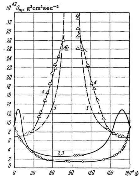
FIG. 3. Angular dependence of  $S_m$  for the new oscillations (curve 4) and for the oscillations connected with Shoenberg's three-ellipsoid model (curves 1, 2, 3).
