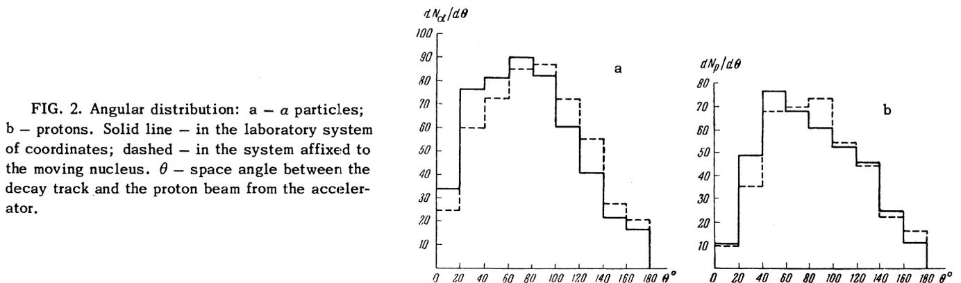
FIG. 2. Angular distribution: a —  $\alpha$  particles; b — protons. Solid line — in the laboratory system of coordinates; dashed — in the system affixed to the moving nucleus.  $\theta$  — space angle between the decay track and the proton beam from the accelerator.
