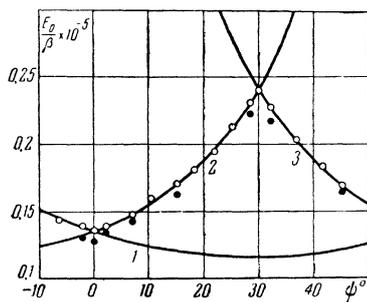
FIG. 2. Variation of oscillation frequency with the angle  $\Psi$  between the magnetic field direction and the diad axis. 1, 2, 3 – theoretical curves derived from Landau's formulae. Experimental data:  $\circ$  – unstressed,  $\bullet$  – with a stress of 340 kg/cm<sup>2</sup>.
