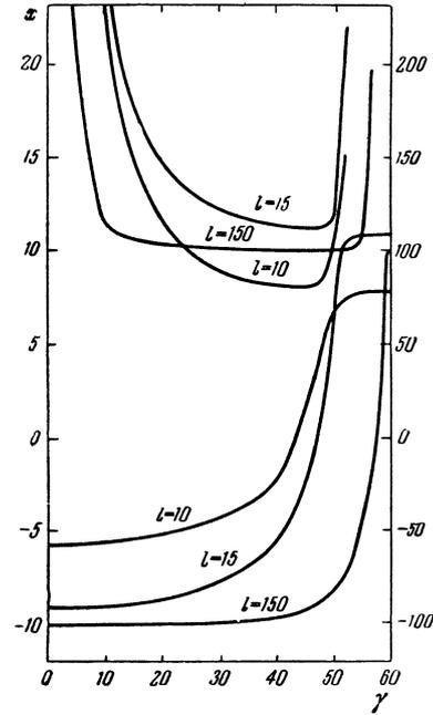
FIG. 1. Nuclear energy as a function of  $\gamma$  and of the quantity  $l$  which determines the coupling of the pair of outer nucleons ( $J = 2$ ) with the nuclear surface deformation. The right hand scale gives the energy for  $l = 150$ .
