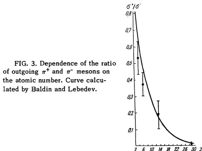
FIG. 3. Dependence of the ratio of outgoing  $\pi^+$  and  $\pi^-$  mesons on the atomic number. Curve calculated by Baldin and Lebedev.
