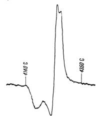
At 850 Mcs there is a clearly pronounced doublets with a distance of  $12 \pm 1$  Gauss between components, produced by the nuclear moment of the hydrogen proton.
