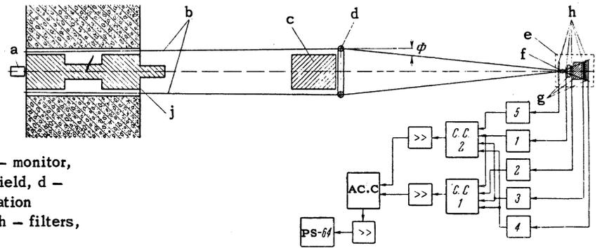
FIG. 1. Overall diagram of the experiment. a – monitor, b – annular neutron beam, c – additional lead shield, d – ring scatterer,  $\phi$  – scattering angle, e – scintillation counters, f – neutron telescope, g – converters, h – filters, j – brass core of the collimator.
