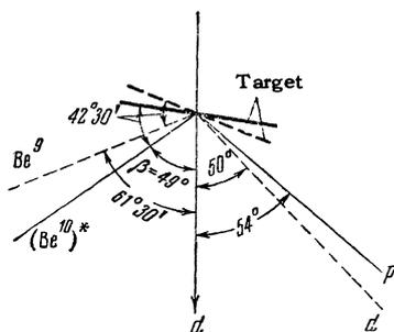
FIG. 4. Angles used in measuring  $\Omega$ .
