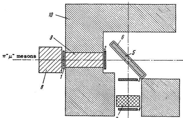
1, 2, 3, 4) scintillation counters; 5) target; 6) magnetizing coil; 7) paraffin filter; 8, 9) aluminum filters; 10) lead shield.
