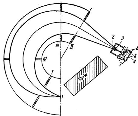
FIG. 1. The electron-optical diagram of the spectrometer. 1) source, 2) entrance slit of the detector, 3) Geiger counter, 4) aluminum target, 5) scintillators, 6) light guides, 7) detector chamber, I-IV) diaphragms.
