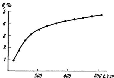
FIG. 2. Dependence of the efficiency  $K$  of the recording system on positron energy.
