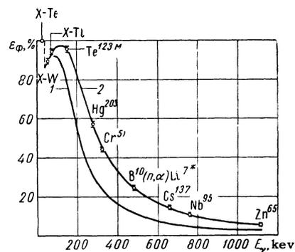
FIG. 1. Photopeak efficiency of spectrometer with NaI (Tl) crystal: 1) crystal with  $h = 10$  mm,  $d = 28$  mm; 2) crystal with  $h = 19.7$  mm,  $d = 30$  mm.
