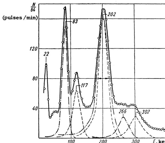
FIG. 3. Spectrum of pulses from  $\text{Ag}^{108}$   $\gamma$  rays, absorbed in  $2.205 \text{ g/cm}^2$  Pb.
