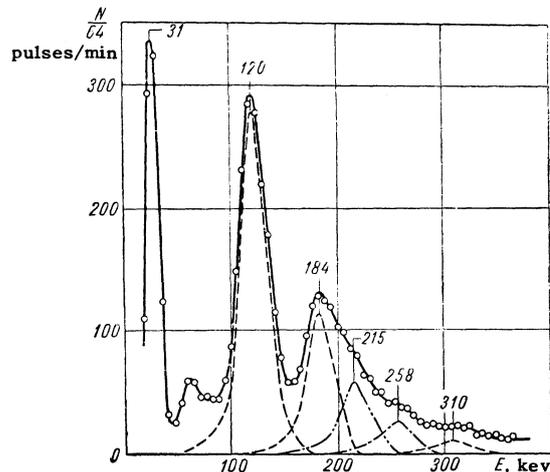
FIG. 6. Spectrum of pulses from  $\text{Cs}^{134}$   $\gamma$  rays absorbed in  $2.205 \text{ g-cm}^2$  Pb.
