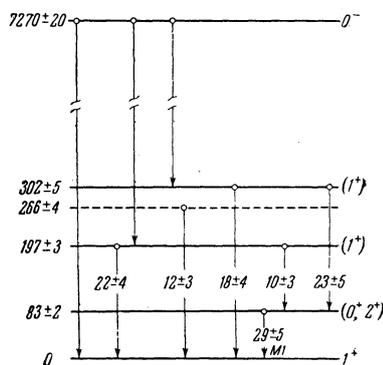
FIG. 4.  $\gamma$ -ray transitions in  $\text{Ag}^{108}$ . The numbers in the breaks in the arrows give the intensities of the transitions in percent per neutron capture, taking account of conversion ( $n_\gamma + k_\gamma$ ).
