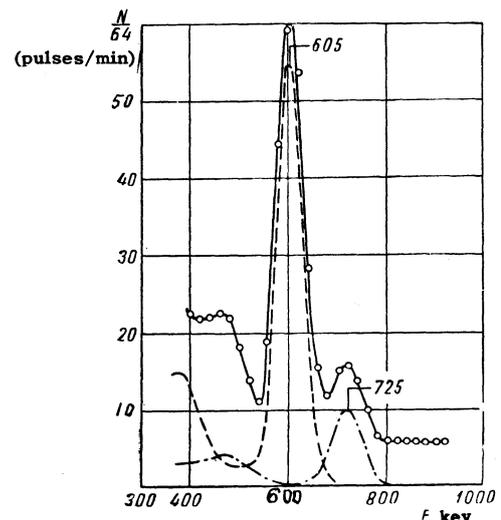
FIG. 5. Spectrum of pulses from  $\text{Te}^{124}$   $\gamma$  rays absorbed in  $4.386 \text{ g/cm}^2$  Pb.
