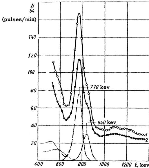
FIG. 2. Spectrum of pulsed from Mo<sup>96</sup> γ rays: 1) measurements without filter, 2) measurements with 5.490 g/cm<sup>2</sup> filter.
