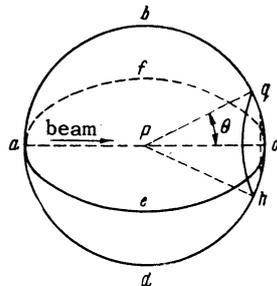
$P$  – point of interaction;  $afce$  – emulsion plane;  $I$  – angle between the planes  $afcPa$  and  $abcPa$ ,  $II$  – angle between the planes  $abcPa$  and  $aPcea$ ,  $III$  – angle between the planes  $aPcea$  and  $aPcfa$ ,  $IV$  – angle between the planes  $aPcda$  and  $aPcfa$ ,  $V$  – solid angle  $qPh$  ( $\theta = 27^\circ$ ),  $VI$  – solid angle ( $4\pi - qPh$ ).
