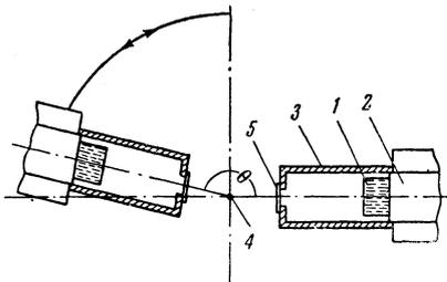
FIG. 2. Arrangement of apparatus for measurement of  $(\gamma, \gamma)$  angular correlation. 1 - stilbene crystal, 2 - FEU photomultiplier, 3 - lead case, 4 - source, 5 - lead filters in front of entrance window in the shielding.
