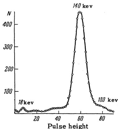
FIG. 4. Soft  $\gamma$ -spectrum from  $\text{Mo}^{99}$ .
