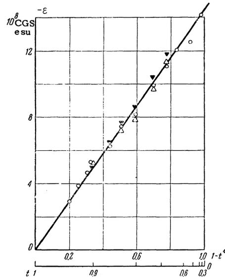
FIG. 5. Variation of the dielectric constant of superconducting cadmium with the relative temperature  $t$ . The three types of symbols represent three series of measurements.
