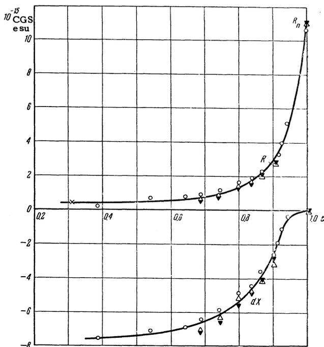
FIG. 4. The surface resistance  $R$  and the changes in the surface reactance  $dX$  of cadmium as a function of the relative temperature  $t = T/T_c$  ( $T_c = 0.56^\circ\text{K}$ ). The three types of symbols represent three series of measurements.
