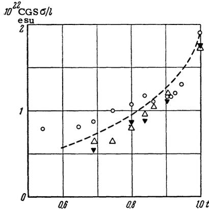
FIG. 6. Variation of the ratio of the conductivity produced by normal electrons to their mean free path with the relative temperature  $t$ . The curve has been drawn approximately through the experimental points. The three types of symbols represent three series of measurements.
