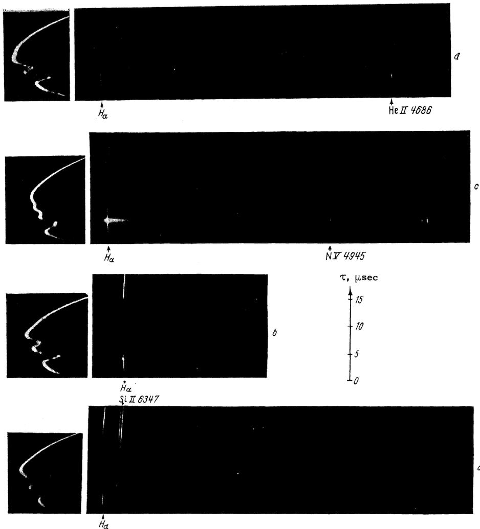
FIG. 2. Spectrogram of the pulsed discharge under various conditions. a) pure hydrogen,  $p_0 = 0.05$  mm Hg; b) pure hydrogen,  $p_0 = 0.1$  mm Hg; c) 95 per cent  $H_2$  plus 5 per cent  $N_2$ ,  $p_0 = 0.05$  mm Hg; d) 70 per cent  $H_2$  plus 30 per cent He,  $p_0 = 0.05$  mm Hg.
