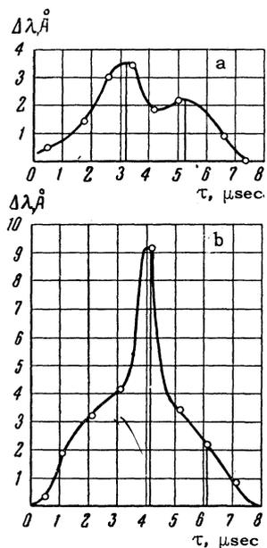
FIG. 3. Time variation of the half-width of the  $H_{\alpha}$  line: a)  $p_0 = 0.05$  mm Hg. b)  $p_0 = 0.1$  mm Hg. The vertical lines denote the first and second contractions of the pinch.
