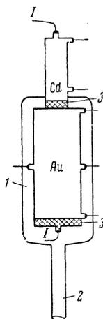
FIG. 1. Mounting of the gold and cadmium specimens.
