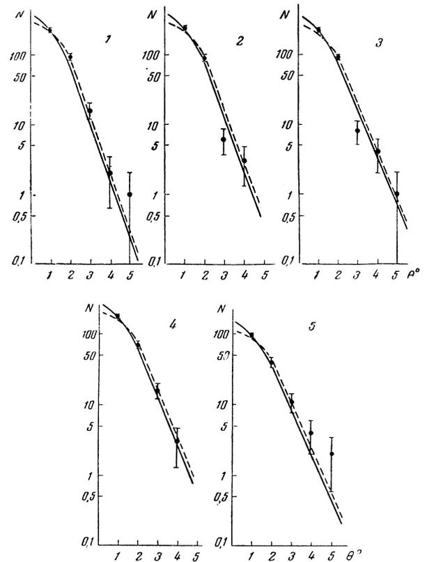
FIG. 2. Angular distributions for the scattering of  $\mu$  mesons in beryllium plates 1-5. Dashed curve: scattering from a point nucleus, solid curve: expected scattering distribution, taking into account the 16% admixture of "hard"  $\mu$  mesons. Mean momentum  $\bar{p}$  is 140, 135, 131, 127 and 125 Mev/c for plates 1 to 5 respectively.
