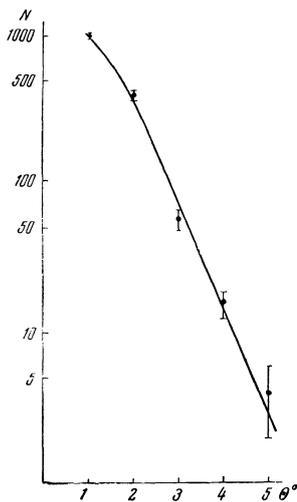
FIG. 3. The total differential cross section for the scattering of  $\mu$  mesons with momentum  $(130 \pm 16)$  Mev/c. The solid curve is a theoretical one, and is the sum of the distributions for each of the plates, taking into account the 16% admixture of "hard"  $\mu$  mesons.
