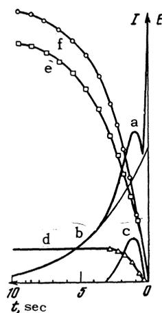
FIG. 6. Analysis of the experimental curve of decrease of viscous emf into two curves, and curves of magnetization obtained by graphical integration.  $H = 0.60$  oersted. a — experimental curve; b — exponential component; c — second component; d — magnetization determined by the second component; e — magnetization determined by the exponential component; f — total magnetization.
