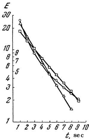
FIG. 5. Dependence of the logarithm of the viscous emf on the duration of the process.  $\circ$ — $H = 0.643$ ;  $\Delta$ — $H = 0.704$ ;  $\square$ — $H = 0.857$  oersted.
