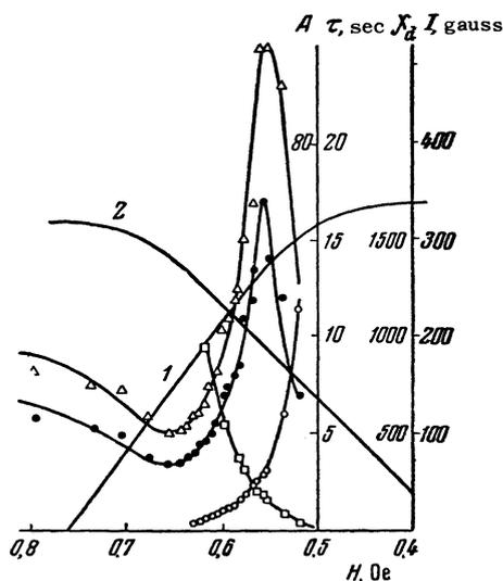
FIG. 2. 1, the back of the hysteresis loop,  $I$ ; 2, curve of the differential susceptibility,  $\chi_d$ ;  $\Delta$  and  $\bullet$ —curves of viscosity,  $\tau_{0.05}$  and  $\tau_{0.01}$ ;  $O$ —curve of the time of appearance of the second maximum of  $\tau$ ;  $\square$ —amplitudes of the second maximum  $A$  for specimen 4.
