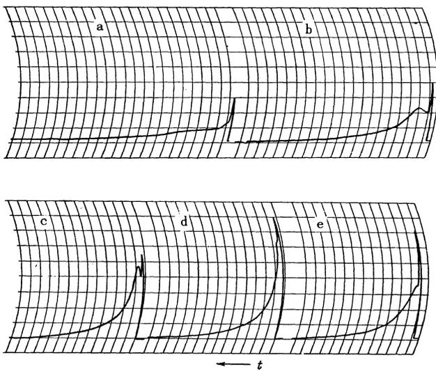
FIG. 1. Curves of the decrease of viscous emf of specimen No. 4. For all curves,  $\Delta H = 0.098$  oersted. a— $H = 0.557$ ; b— $H = 0.588$ ; c— $H = 0.618$ ; d— $H = 0.630$ ; e— $H = 0.704$  oersted.
