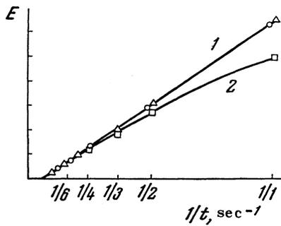
FIG. 4. Dependence of the viscous emf of specimen 4 on the reciprocal of the duration of the process.  $\circ$ — $H = 0.630$ ;  $\Delta$ — $H = 0.636$ ;  $\square$ — $H = 0.643$  oersted.
