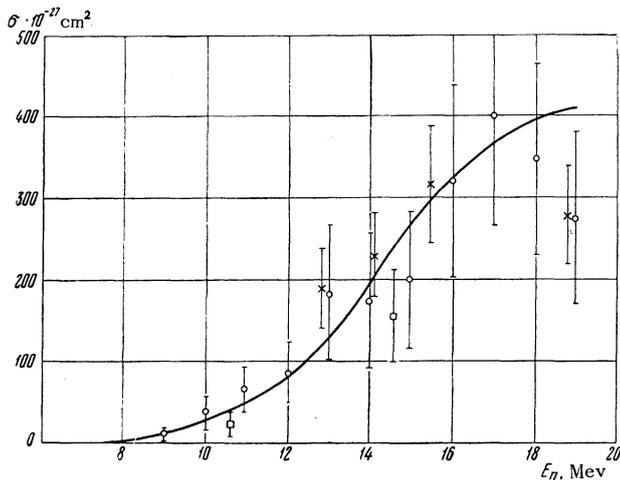
FIG. 1. The effective cross section for the decay of  $C^{12}$  into three  $\alpha$  particles when bombarded by fast neutrons.  $\circ$ —data of the work reported in this paper,  $\times$ —data from Ref. 1,  $\square$ —data from Ref. 2. Solid curve—the cross section according to Sachs' semi-empirical formula,<sup>4</sup> with  $R = 0.88$ ,  $a = 1.06$ .
