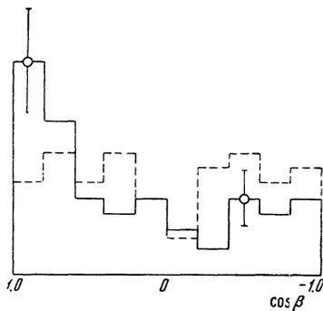
**FIG. 2.** The angular distribution of the inelastically scattered neutron in the center-of-mass system. Solid curve —  $E_n = 18 - 19$  Mev, dashed curve —  $E_n = 13 - 14$  Mev.
