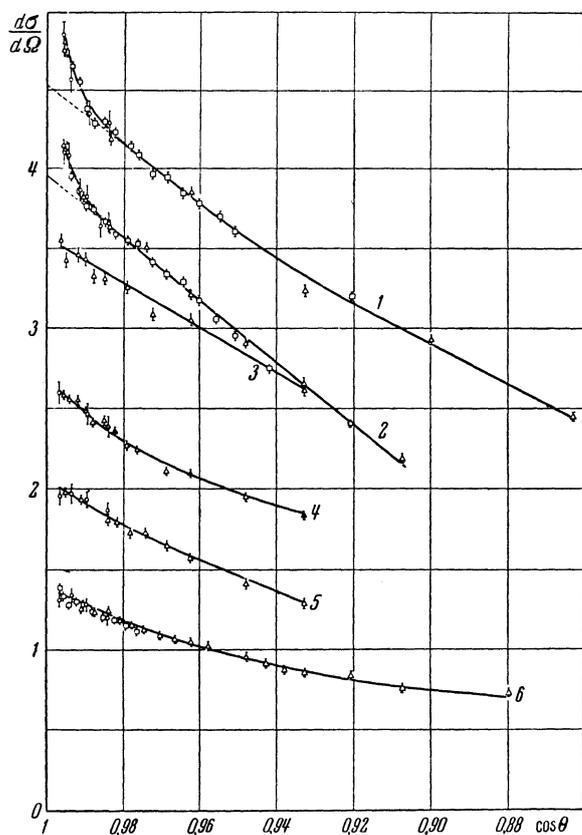
FIG. 3. Experimental results. All experimental points are corrected for the Schwinger scattering cross section. Curves 1, 2, 3, 4, 5, and 6 refer to Pu, U, Sn, Pb, Bi, and Cu, respectively. The vertical scales for curves 4 and 5 are decreased by factors of 1.5 and 2.
