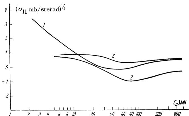
FIG. 4. Energy dependence of the polarization correlation, as measured with scattering planes parallel. 1. Correlation for  $\theta = 20^\circ$ ; 2. Total and nuclear correlation for  $\theta = 90^\circ$ ; 3. Nuclear part for  $\theta = 20^\circ$ .
