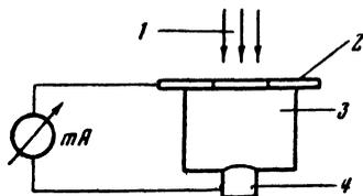
FIG. 2. 1—light, 2—nickel collar, 3— $n$ -type germanium, 4—indium.
