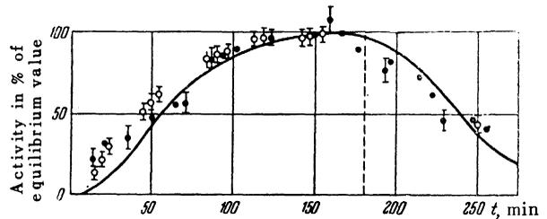
FIG. 5. Dependence of neutron and  $\gamma$  activity of radon on time.  $t=0$ —clean ampoule filled with radon;  $t=180$  min.—radon pumped out.  $\circ$ —Rn in glass tap (for  $\gamma$  rays).  $\square$ —purified Rn in a Pt ampoule (for neutrons); solid curve as computed for RaC.
