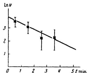
FIG. 6. Time dependence of the neutron activity of preparations enriched with RaC''
