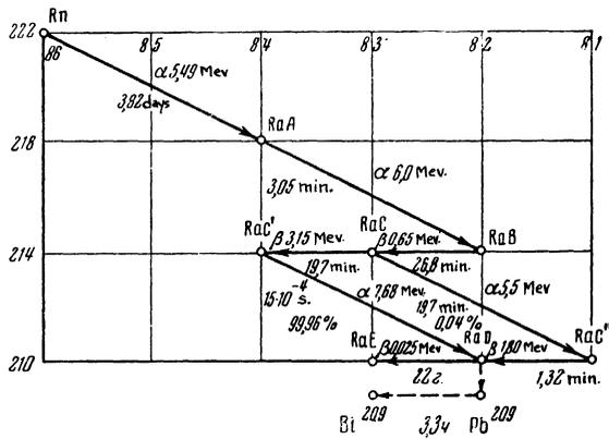
FIG. 4. Radioactive decay scheme for radon disintegration
