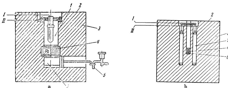
FIG. 1. Experimental arrangement for measuring neutron activity. I—lead to the linear amplifier, II—lead to the high voltage source; 1—ionization chamber, 2—screen, 3—paraffin block, 4—lead filter, 5—trap, 6—chamber with source, 7—neutron counter, 8—ampoule with source.
