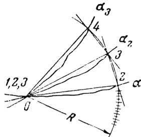
FIG. 2. Eye-piece scale, used for measuring the angles of magnetic deflection and multiple scattering of particles.
