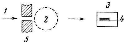
FIG. 1. Sketch of the experiment. 1,  $\gamma$ -rays. 2, Magnetic field of 7000 gauss. 3, Pulsed magnetic field generator. 4, Nuclear emulsion. 5, Collimator.
