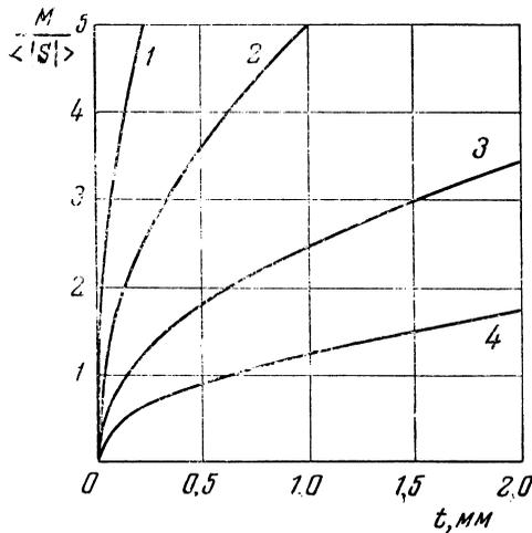
FIG. 3. Results of a calculation of the ratio of the magnetic deflection  $M$  to the multiple scattering angle  $\langle |S_i| \rangle$  for an electron or positron. The abscissa is the length of the observed track. Curves are shown for various values of  $H$ . 1,  $H = 4.8 \times 10^5$ . 2,  $H = 2.4 \times 10^5$ . 3,  $H = 1.2 \times 10^5$ . 4,  $H = 0.6 \times 10^5$  gauss.
