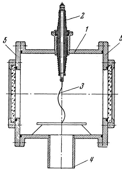
FIG. 1. Diagram of a vacuum chamber.
