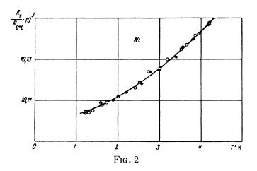
of iron and nickel, which distinguishes them from other metals and which manifests itself in the presence of a linear term in the temperature dependence of the resistance.
