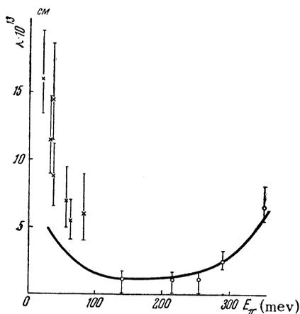
FIG. 2. Dependence on energy of the meson path  $\lambda$  in the nuclear matter. [O - experimental points obtained by the optical model in the present work;  $\times$  - works cited in reference 11; solid curve computed without allowance for the Pauli principle from cross section data for scattering of  $\pi$ -mesons by nucleons.
