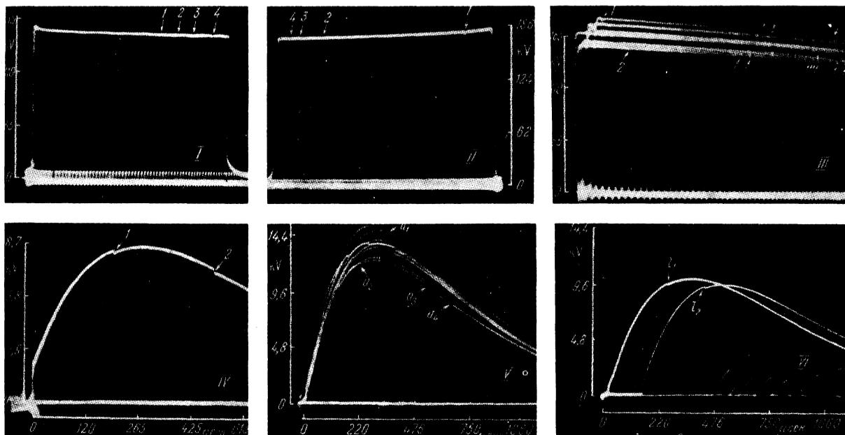
FIG. 2. Oscillographs of the voltage behavior at breakdown and during the prebreakdown period in transformer oil, castor oil, xylene, and paper impregnated with transformer oil.
