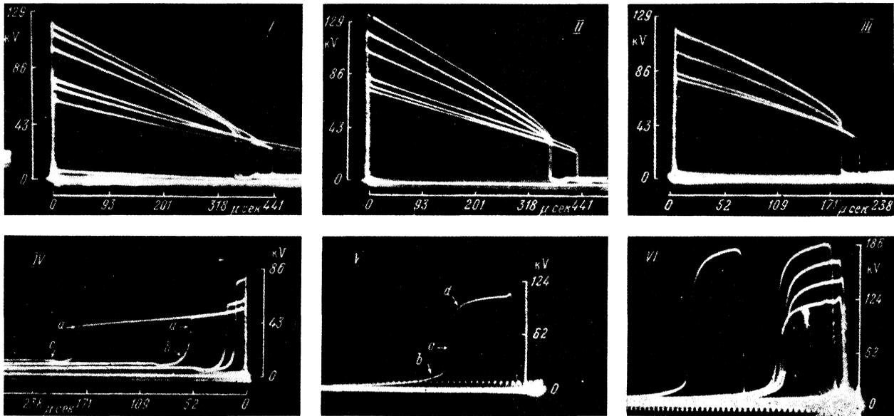
FIG. 3. Oscillographs of the voltage behavior at breakdown and during the prebreakdown period in distilled water.
