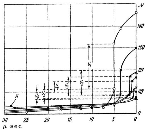
FIG. 4. Curves showing the decay of the voltage in the formation of a discharge in distilled water (positive point and plane);  $U_1 = 84$ ;  $U_2 = 44$ ;  $U_3 = 34$ ;  $U_4 = 22$ ;  $U_5 = 16$ ;  $U_6 = 12$  kV
