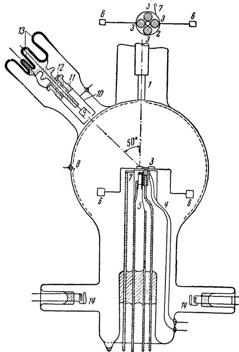
FIG. 1. Vacuum tube device. 1 - electron gun; 2 - platform; 3 - objects under investigation; 4 - thermocouple; 5 - heater filament; 6 - small iron rods imbedded in glass; 7 - locking spring; 8 - collector; 9 - Faraday cylinder; 10 - cylinder with diaphragm; 11 - quartz tube; 12 - protective cylinder; 13 - ceresin; 14 - getter.
