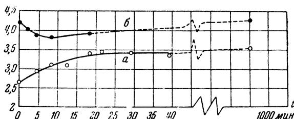
FIG. 4. Effect of change in temperature on the intensity of reflection: a - from the (111) plane of copper oxide; b - from the (110) plane of copper oxide.
