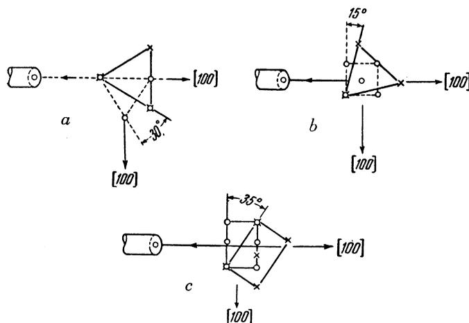
FIG. 3. Schematic of the mutual dispositions of the lattices of copper oxide and copper. The broken line represents the lattice of copper, and the solid line the lattice of  $\text{Cu}_2\text{O}$ . The primary cluster of electrons falls on the monocrystals from above. The arrows show the direction of the dispersed electrons to the Faraday cylinder. The zones of the copper lattice are shown in each drawing.
