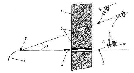
FIG. 1. Experimental Arrangement.  $1 - \text{Concrete shield}; 2 - \text{Collimators}; 3 - \text{Target (Be)}; 4 - \text{Neutrons}; 5 - \text{Protons } (E_p = 580 \text{ mev}); 6 - \text{Sample}; 7 - \text{Telescope}; 8 - \text{Bi- Chamber}; 9 - \text{Detecting telescope}; 10 - \text{Filter}; 11 - \text{Scatterer}$
